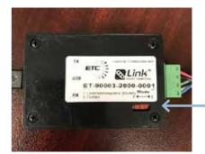
Ensure the RX switch found on the back of your Link Kit is set to position 2 for Cyclops. Open ETC Vision and navigate to the "Setup" tab and select "Cyclops" as the device type you are connecting to from the Device dropdown.
