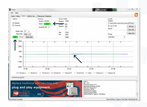
Simply move any ferrous object past the Cyclops to simulate a plunger arrival, and you will see the signature of the introduced change causing the Sample reading to exceed the thresholds.
