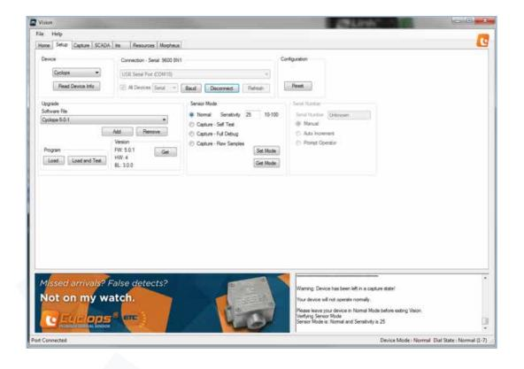
Once you have confirmed the Sensor Mode is "Normal" via the pop up notification on your screen, you can "Disconnect the USB Serial Port connection, and put the sensor back into operation in the field.
