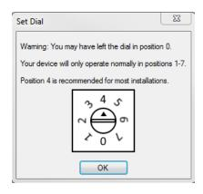
You will also see a reminder to ensure the Manual Sensitivity dial is set to a value other than "O" before going back into operation in Normal mode.
